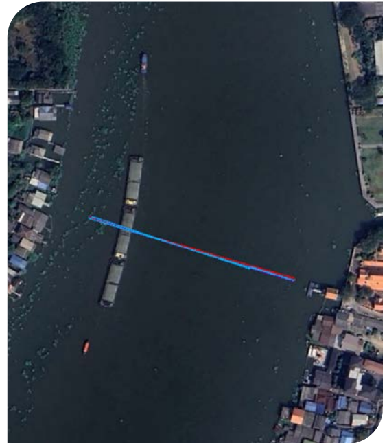
Figure 1. Transects (blue – GNSS track and red – Bottom Track) performed by Flow Seeker across a channel more than 200 meters wide.
