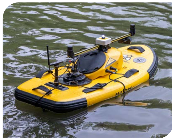
Surfbee Flow Seeker equipped with a SonTek-RS5.
