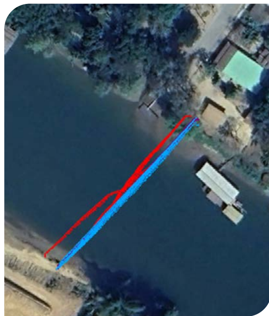
Figure 3. Transects (blue – GNSS track and red – Bottom Track) performed by Flow Seeker across a channel with highly variable flow. Note the deviation in bottom track ship tracks, indicating a moving bed at this site.
